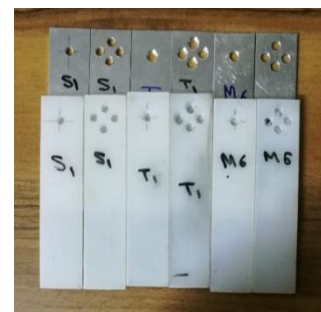
Figure 2. First group of examination specimens Note: (S) cylindrical, (T) double-conical, (M) toothed cylindrical.
