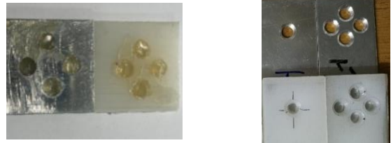
(b) Double-conical resin rivet
