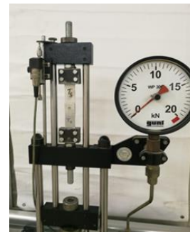
Figure 1. Multi-test machine showing the test specimen before loading
