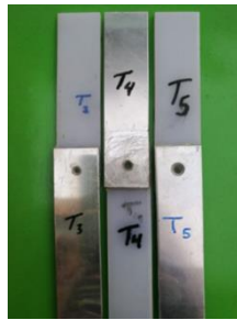
Figure 4. Bonding of the single-hole, double-conical joint using unsaturated polyester resin (UPR)
