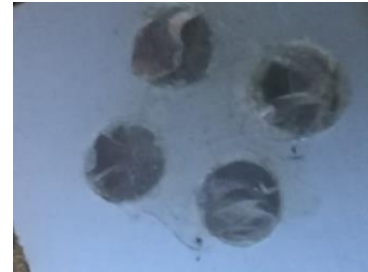
Figure 5. Cross-sectional morphology of the fractured four-hole aluminum–high-density polyethylene (Al-HDPE) hybrid joint after shear testing, showing internal resin filling and mechanical interlocking
