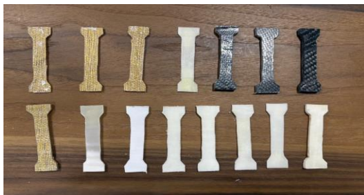
Figure 6. Compression test specimens
