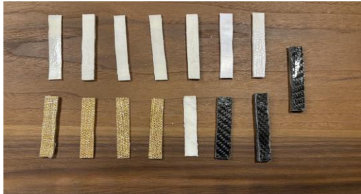
Figure 5. Impact test specimens
