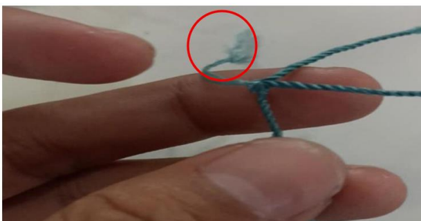
Figure 2. Representative post-failure netting specimen showing catastrophic tensile rupture localized within the mesh legs (red circle), while the knot junction remains intact
