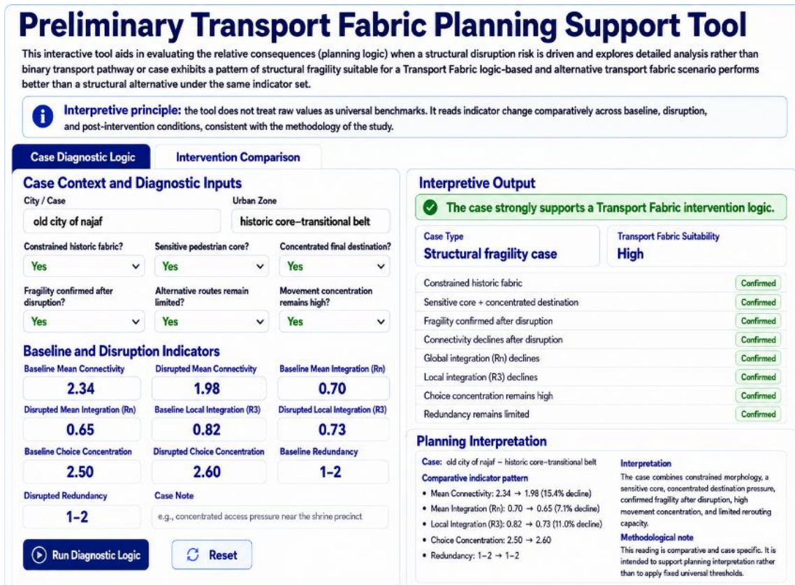
Figure 11. Preliminary interface of the Transport Fabric planning support tool based on the baseline and critical-node disruption values
