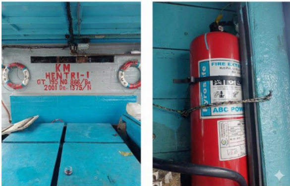
Figure 3. Firefighting and survival equipment observed onboard (portable extinguishers and lifebuoy arrangement)
