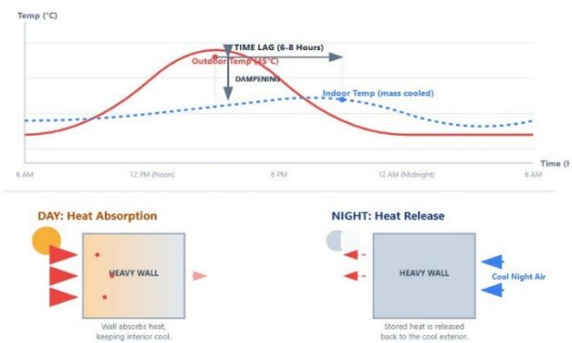
Figure 2. Thermal mass: The time lag effect
