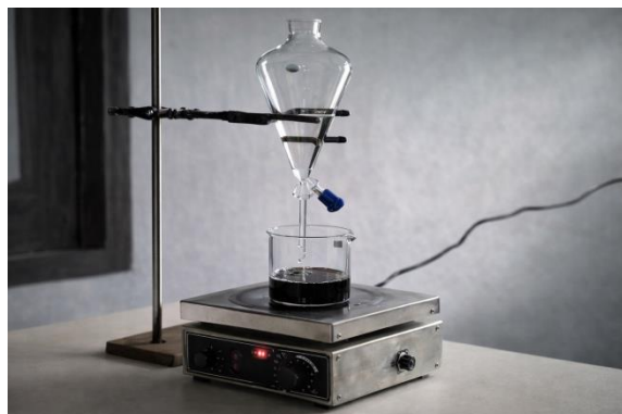
Figure 4. Polyaniline (PANI) preparation
