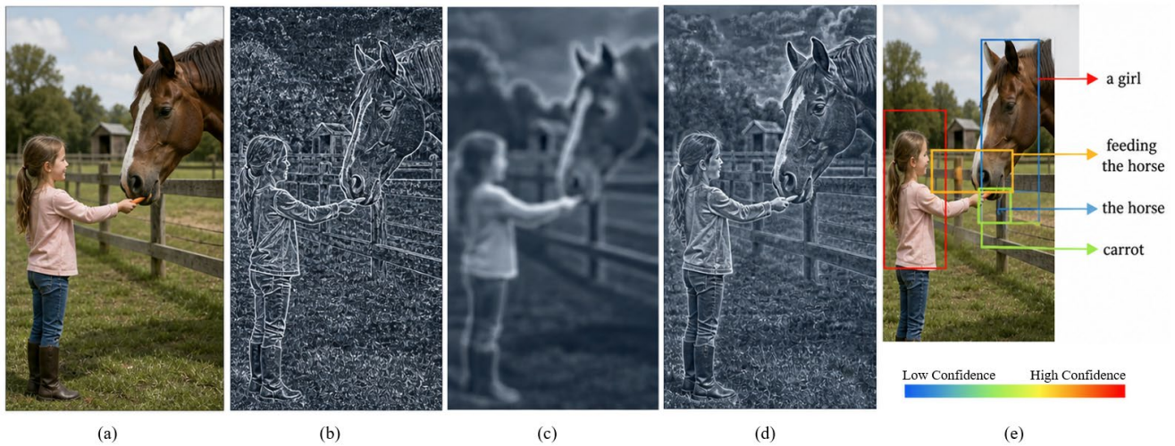
Figure 7. Example of multi-granularity visual feature fusion and alignment effect of the proposed method: (a) Original input image; (b) Local texture features extracted by ConvNeXt only; (c) Global semantic features extracted by Swin Transformer only; (d) Enhanced features after adaptive gated fusion; (e) Visual-semantic alignment arrow diagram
