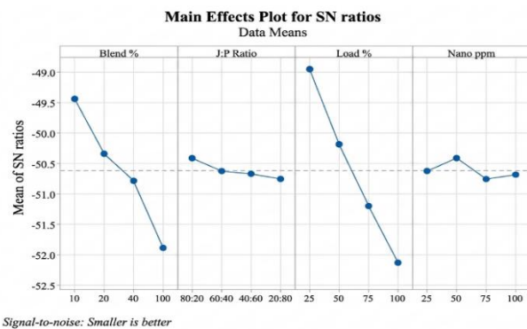
Figure 5. Main effects plot of S/N ratios for NO x emissions
