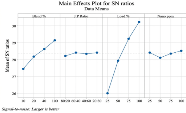
Figure 3. Signal-to-noise ratio plot for brake thermal efficiency (BTE)
