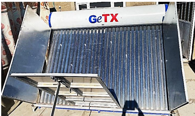
Figure 3. Test rig with three enhancements
