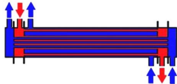
Figure 13. The coaxial with shell-and-tube heat exchanger's (CWST) longitudinal section showing the hot (in red) and cold (in blue) fluids
