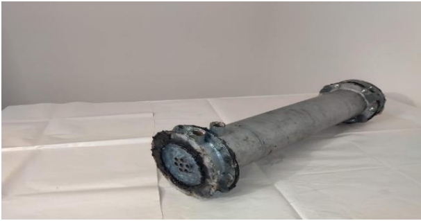
Figure 8. Coaxial with shell-and-tube heat exchanger (CWST) without last distributors
