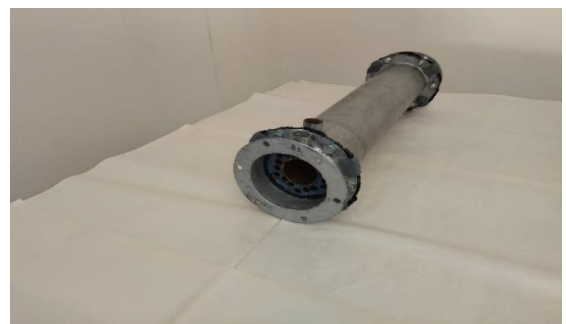
Figure 7. Coaxial with shell-and-tube heat exchanger (CWST) without the last distributors, their tube sheets, and the tubes connected to them
