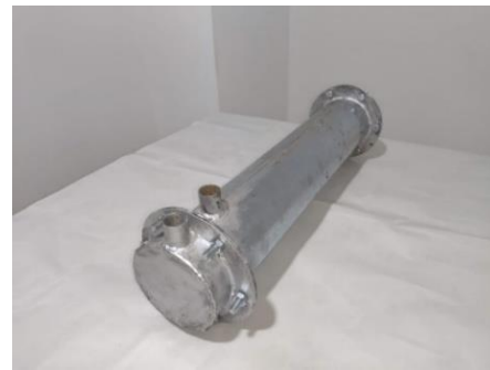
Figure 3. Shell-and-tube heat exchanger (STHE) with distributors
