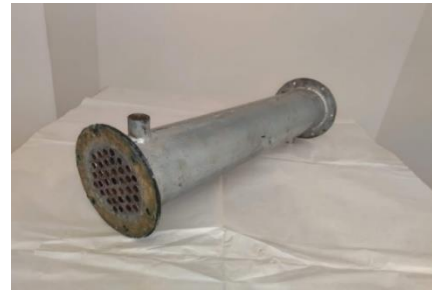
Figure 2. Shell-and-tube heat exchanger (STHE) without distributors
