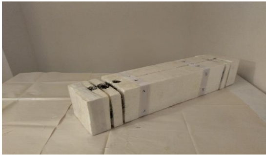
Figure 10. Coaxial with shell-and-tube heat exchanger (CWST) insulated with polystyrene
