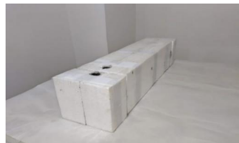
Figure 4. Shell-and-tube heat exchanger (STHE) insulated with polystyrene
