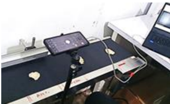
Figure 3. Setting for real-time classification of melinjo chips
