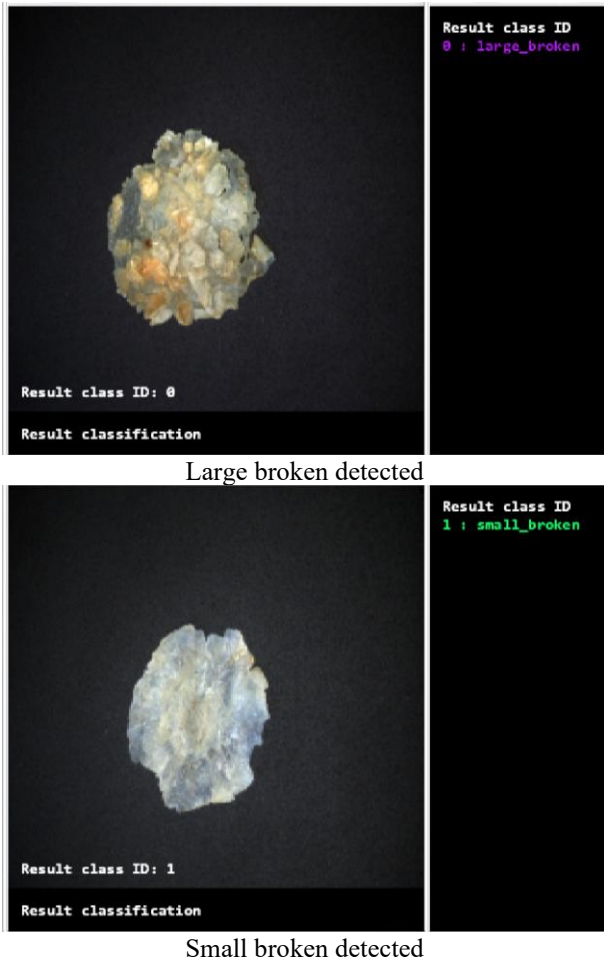
Figure 7. Example of real-time classification of a melinjo chips sample using MVTec Halcon software
