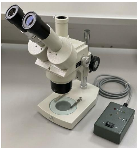
Figure 2. Optical microscope (Meiji Techno EMZ-5 / EMZ-8 Stereo Microscope) used for microstructural analysis
