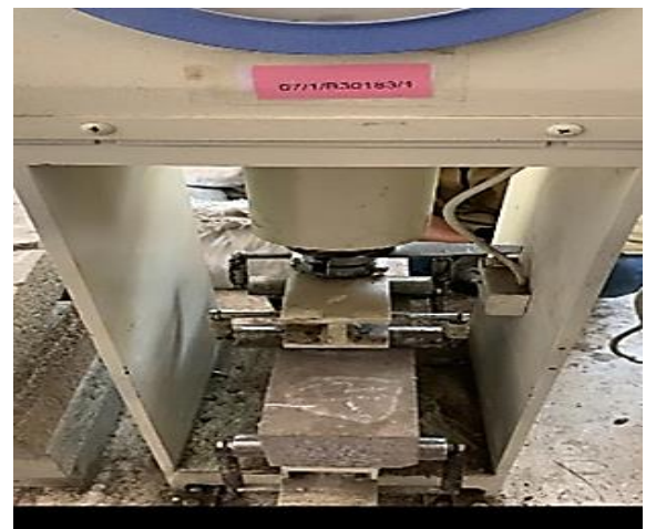
Figure 9. Flexural strength test
