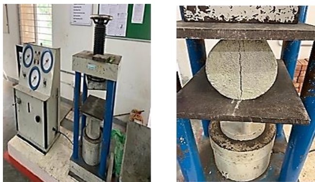
Figure 7. Split tensile strength
