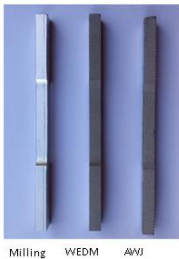
Figure 2. The macroscopic surface appearance of tensile test specimens
