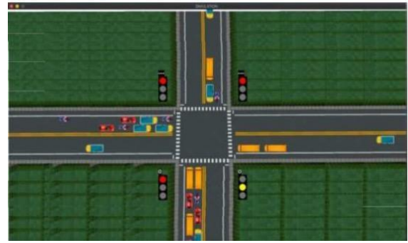
Figure 4. Pygame-based traffic simulation environment for a 4-way intersection
