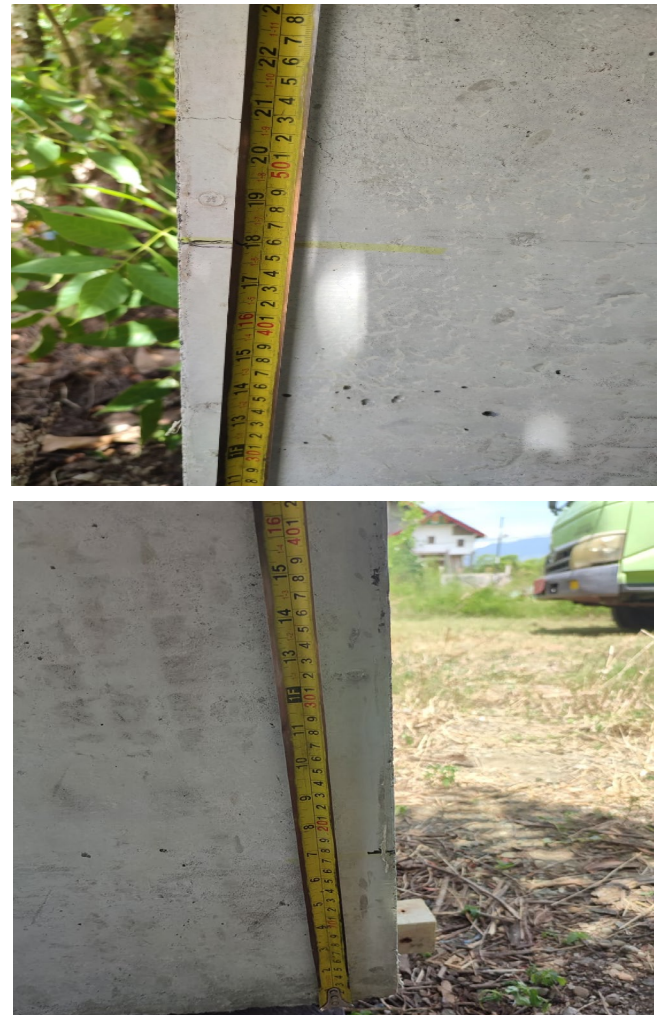
Figure 6. Draft measurement during pontoon testing
