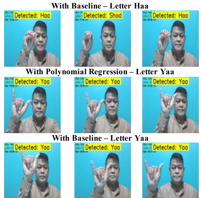
Figure 4. Representative real-time detection results comparing baseline and polynomial regression models for Hijayah letter recognition
