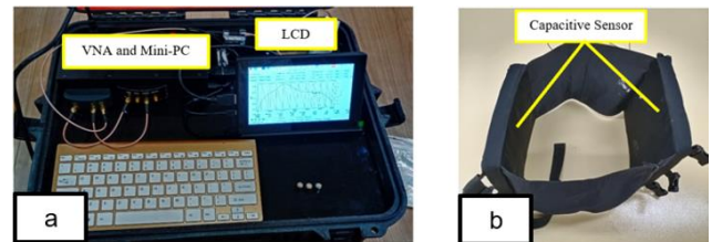
Figure 1. Prototype of ECT-S system (a) DAS component and (b) Belt-shaped capacitive sensor
