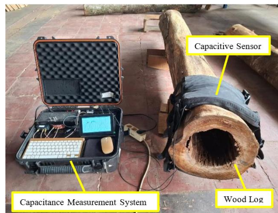
Figure 3. Experimental setup for measuring wood electrical characteristics in a wood log
