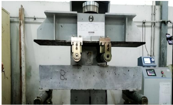
Figure 5. Test setup of beam B0
