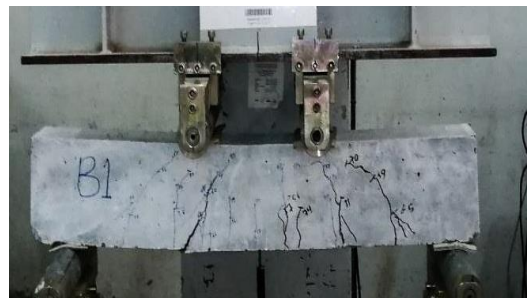
Figure 11. The patterns of cracks for the beam B1
