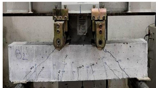
Figure 12. The patterns of cracks for the beam B2
