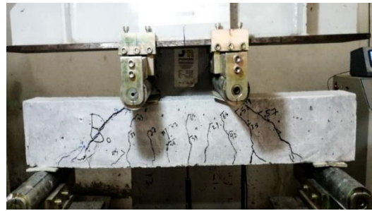
Figure 10. The patterns of cracks for the beam B0
