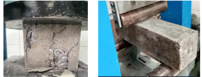
Figure 6. Mechanical properties testing (a) compression test specimens, (b) three-point bending test specimen
