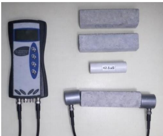
Figure 5. Ultrasonic testing of concrete specimens
