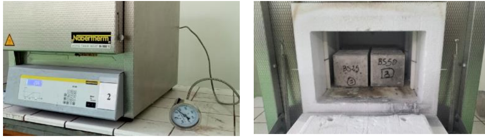
Figure 4. Heating of test specimens inside the furnace
