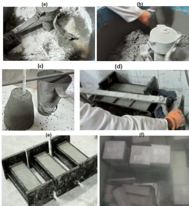
Figure 2. Test specimen preparation (a) mechanical mixing, (b) mixing of the concrete in the mechanical mixer, (c) slump test for workability of fresh concrete, (d) preparation of concrete specimens in moulds on a vibrating table, (e) concrete specimens in moulds, (f) the specimens in the water
