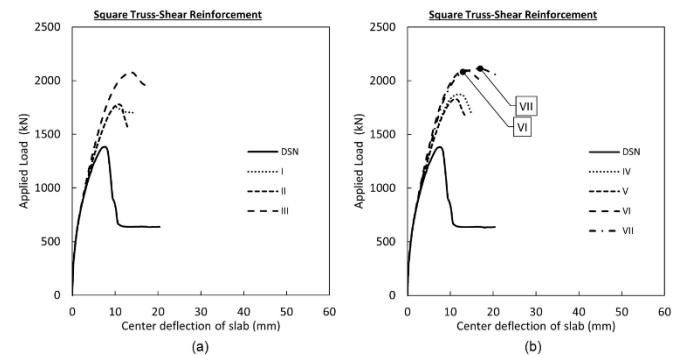
Figure 13. Load-deflection response of the slab models in Group 4
