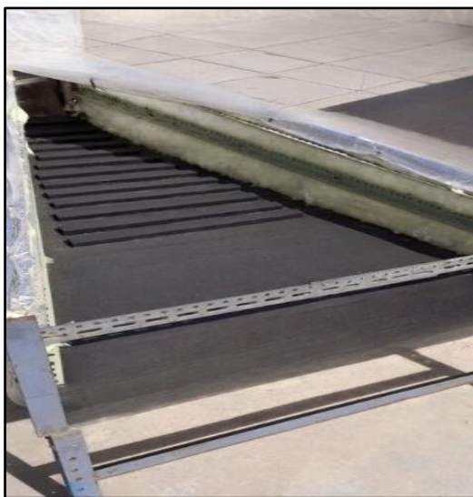
Figure 6. Plate of the test section with 12 flat ribs along the absorber aluminium plate
