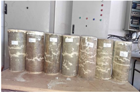
Figure 2. Confined concrete specimens
