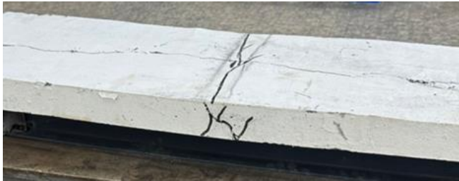
Figure 11. Crack pattern of specimen CRB5
