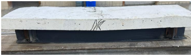
Figure 16. Crack pattern of specimen CRB6
