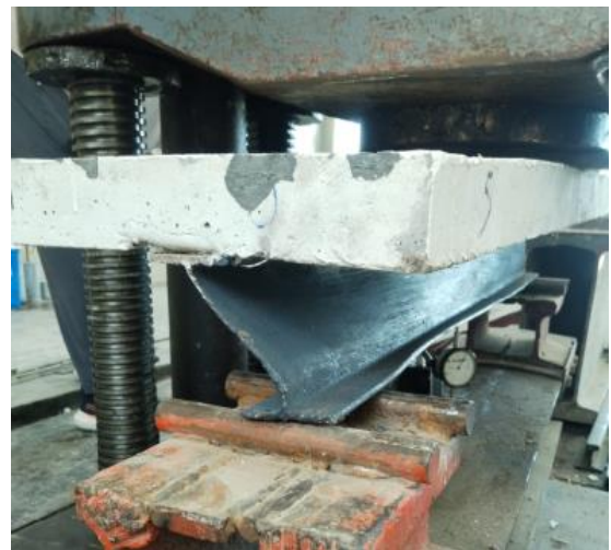
Figure 17. Crack pattern of specimen CRB6
