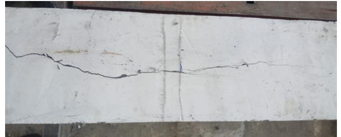
Figure 13. Longitudinal cracks of specimen CRB4
