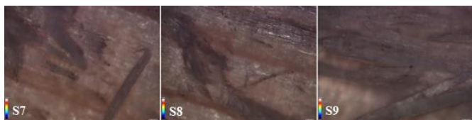
Figure 16. Profilometry images of moisture-conditioned spruce wood samples (S7–S9) after three-point bending tests illustrating microcracks and fiber pull-out
