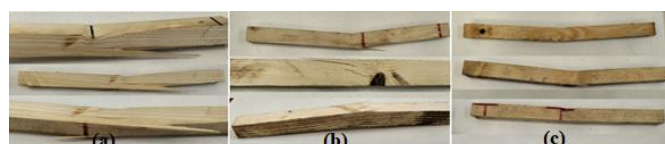
Figure 10. Spruce wood samples after three-point bending tests for (a) Oven-dried, (b) Air-dried, and (c) Moisture-conditioned
