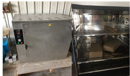
Figure 2. Sample preparation: Oven drying and pretest conditioning
