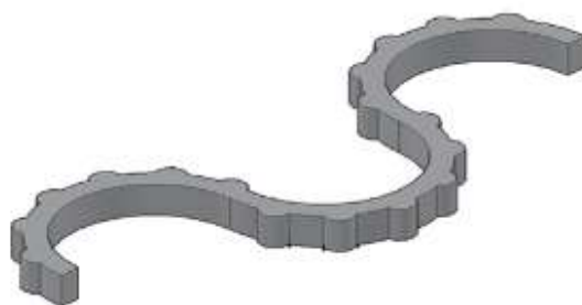
Figure 10. A schematic display of 3D geometric parameters of a serpentine microchannel with fan-shaped reentrant cavities [43]
