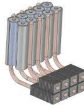
Figure 13. Battery pack PCM cooling
