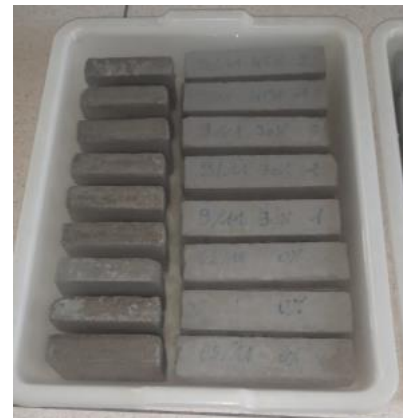
Figure 9. Mortars placed in a container of water
