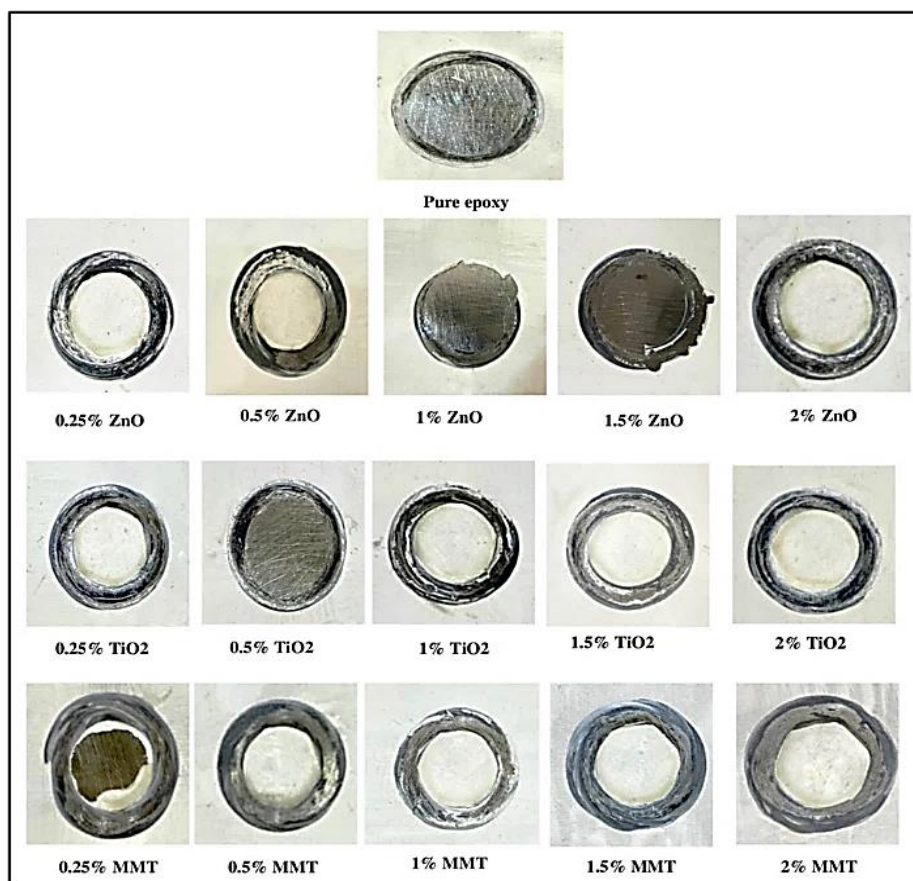
Figure 8. Image of adhesive failure demonstrated on the steel substrate
