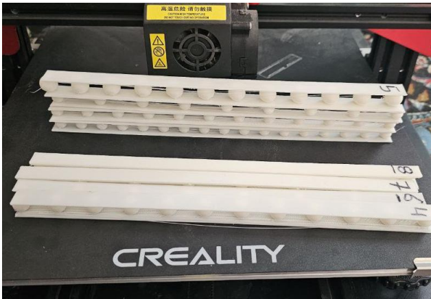
Figure 4. Samples sandwich beam with spherical core used in experimental work
