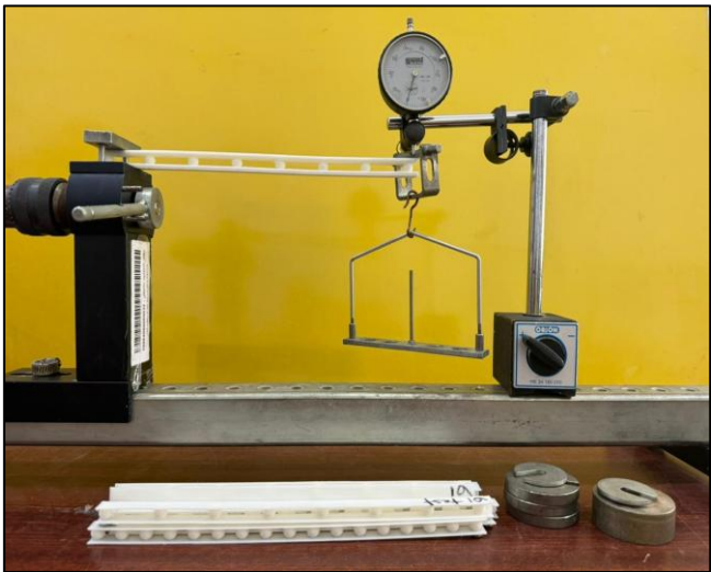
Figure 5. The experimental setup of the static deflection test
