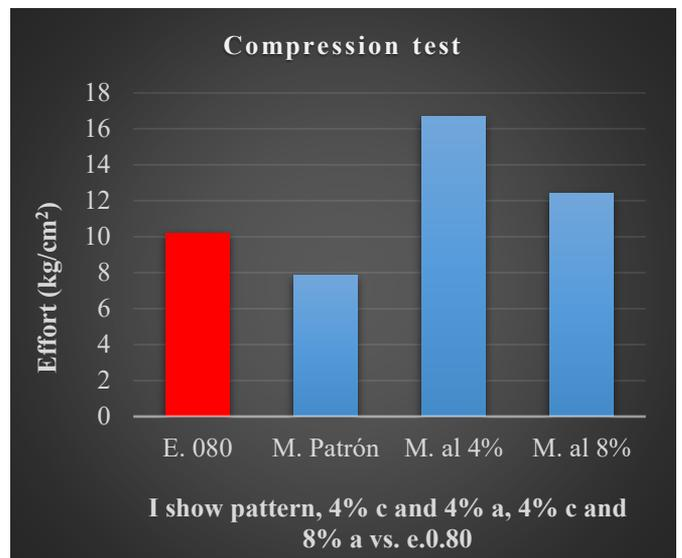
**Figure 1.** Compressive strength – standard sample summary chart, and addition of 4% kaolin and 4%–8% sawdust
