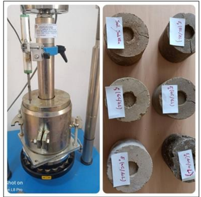
Figure 5. CBR test apparatus
