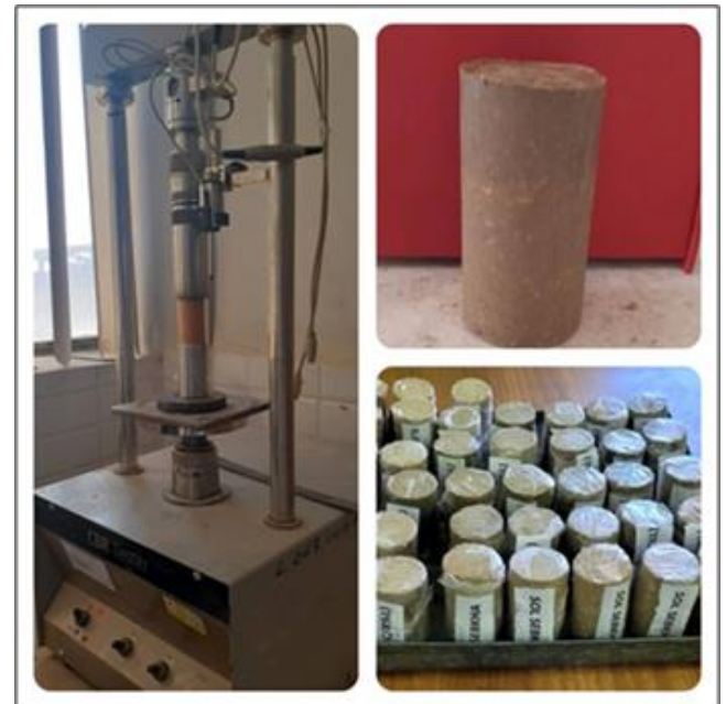
Figure 6. UCS test apparatus
