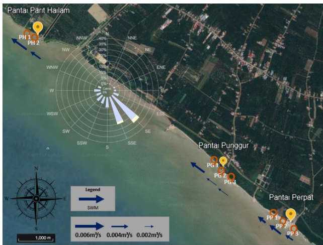
Figure 11. Illustration of dominant wave and wind directions driving longshore sediment transport
