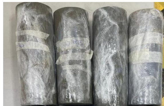
Figure 8. Cylindrical soil samples were prepared for the bulk density test
