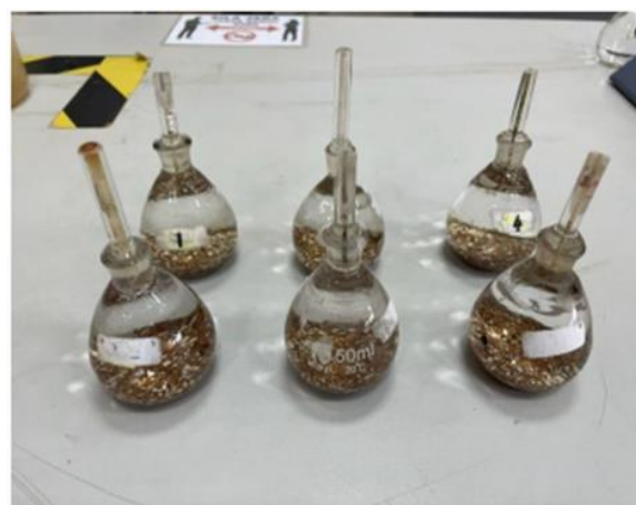
Figure 7. Soil sample and distilled water in pycnometers
