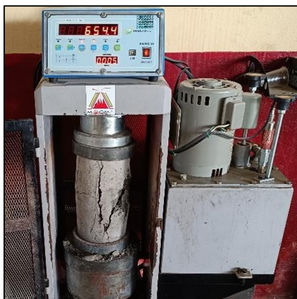
Figure 8. Breakage of concrete specimens
