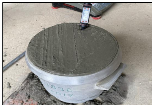
Figure 5. Concrete temperature test
