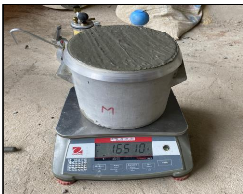
Figure 4. Unit weight test
