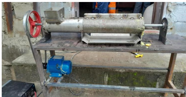
(b) Complete assembly of the solar-powered fruit juice extractor
