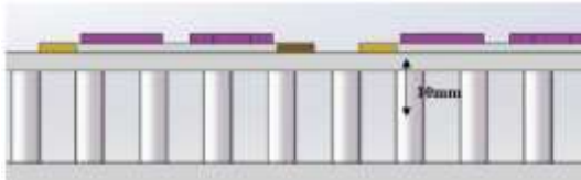
(a) Cross section of traditional bifurcated spoiler column
