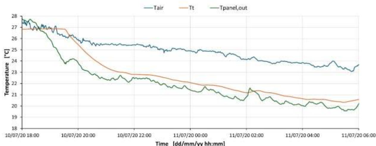
Figure 10. Outdoor temperature ( T_{air} ), outlet temperature of working fluid ( T_{panel,out} ), and tank temperature ( T_t ) for a full scale system
