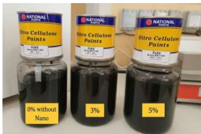
Figure 2. Mixture of black paint with CuO nanomaterial
