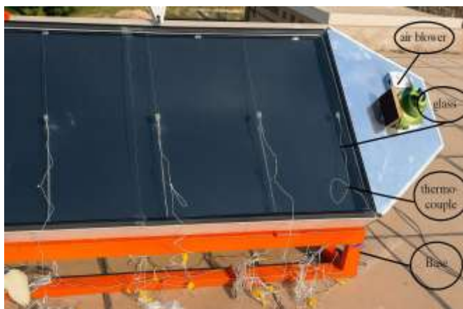
Figure 1. Displays the experimental set-up
