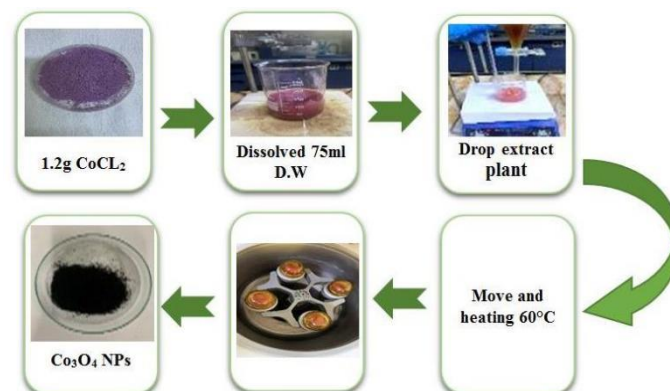
Figure 2. The steps to prepare the pure \text{Co}_3\text{O}_4 NPs using Capparis spinosa fruits using a green approach
