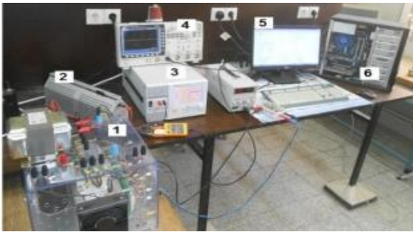
Figure 1. Photograph of the emulator used for data collection: 1) buck converters, 2) load, 3) programmable power source, 4) scope, 5) ControlDesk, 6) DS1104 platform [20]
