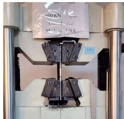
Figure 4. Universal testing machine used for tensile testing of RFW specimens
