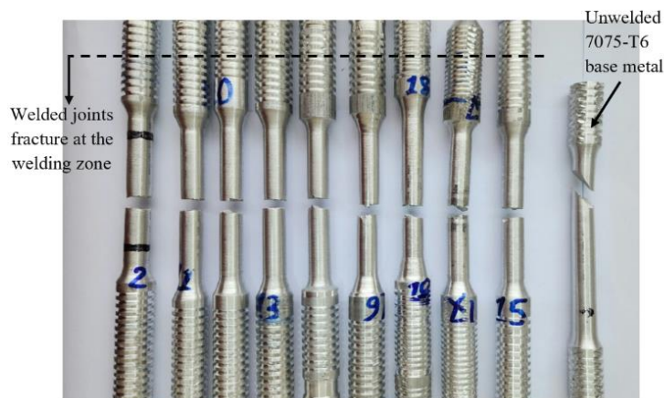
Figure 6. Tensile specimens after fracture show consistent weld zone failure
