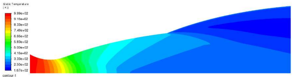
Figure 26. Static temperature contour: T_0 = 1000 K (High-Temperature gas model)
