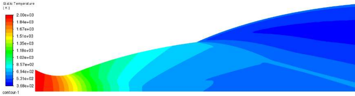
Figure 27. Static temperature contour: T_0 = 2000 K (Perfect gas model)
