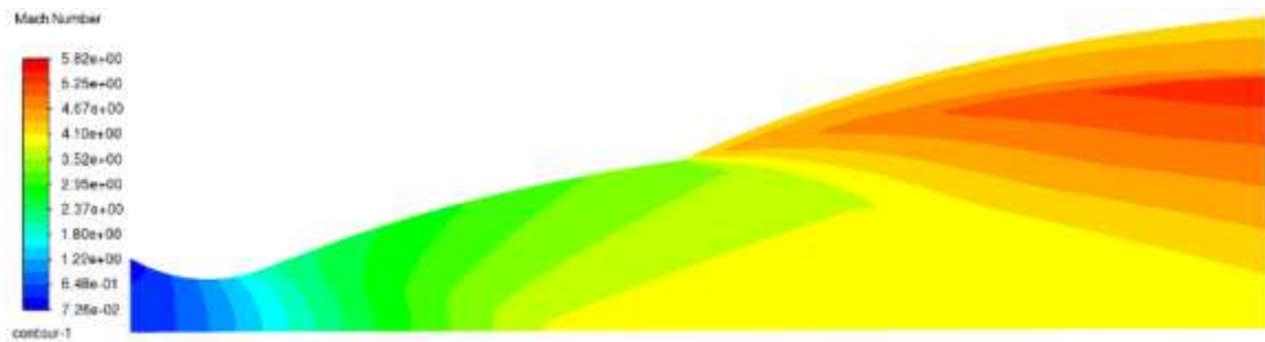
Figure 20. Mach number contour: T_0 = 3000 K (High-Temperature gas model)
