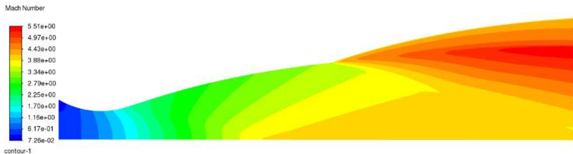
Figure 17. Mach number contour: T_0 = 243 K (Perfect gas model)
