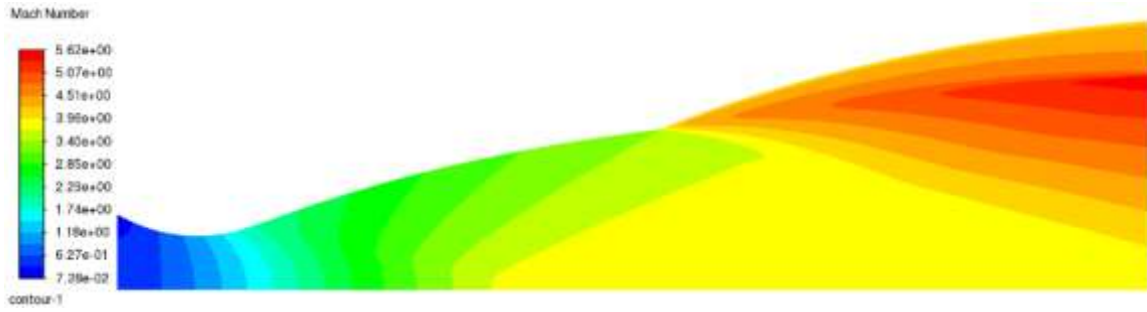
Figure 18. Mach number contour: T_0 = 1000 K (High-Temperature gas model)
