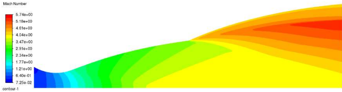
Figure 19. Mach number contour: T_0 = 2000 K (Perfect gas model)
