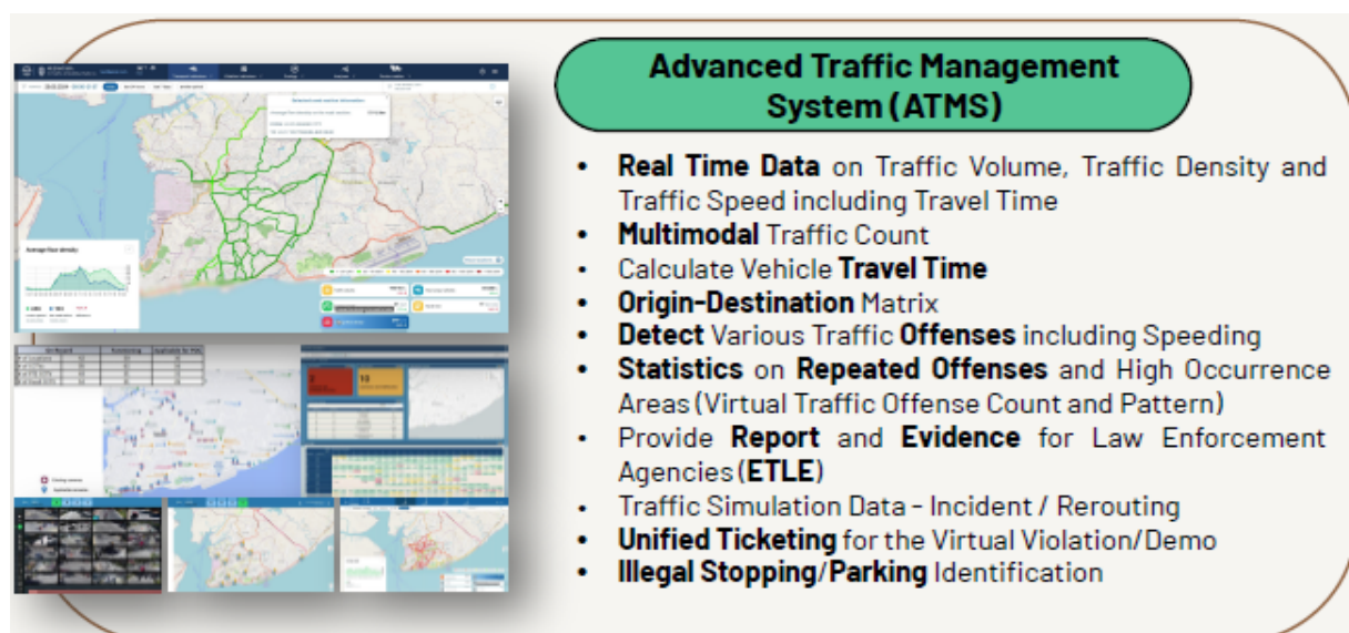
Figure 5. Overview of the advanced traffic management system (ATMS) features in Nusantara [58]
