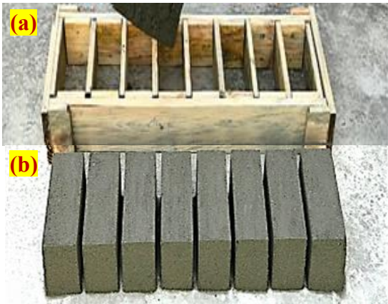
Figure 4. Presentation of (a) wooden mold, (b) cast composites
