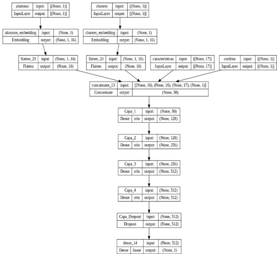
Figure 5. Architecture of the neural network used for elective course prediction
