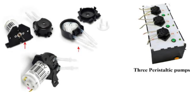
Figure 3. Components of a lab-built peristaltic pump
