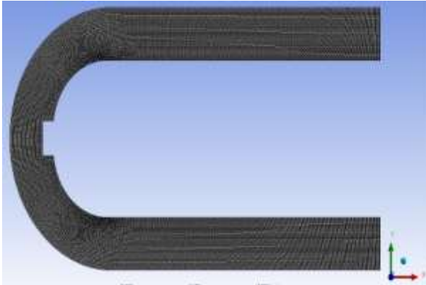
Figure 3. Mesh generation of single and double domains
