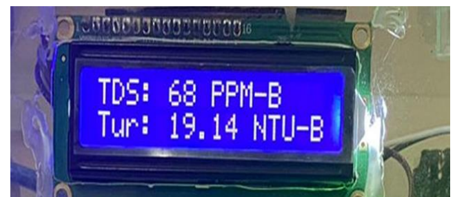
Figure 11. LCD displays sensor value
